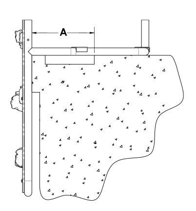
RIM FLOW GUTTER DIMENSION A REQUIRED
